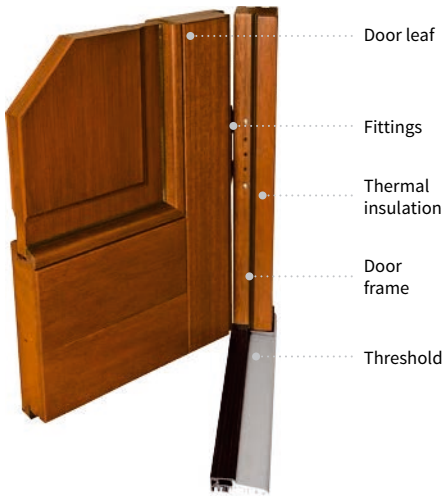
Cross-section of standard door
